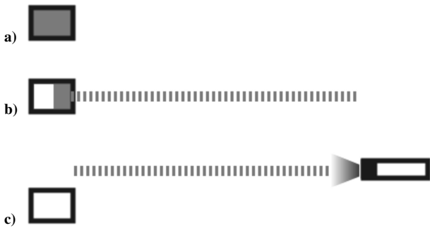
Fig. 1 Mass stream propulsion concept viewed in the reference frame of a transit craft. In a) the transit craft (filled rectangle) carries the mass that is to be released into a stream, b) the mass is released into the stream (gray dashed line) over a period of days, and c) the stream strikes an ablator on the propelled spacecraft (black rectangle). The transit craft shifts to the side to avoid a collision with the propelled craft.
